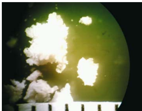
Fig. 1 Microscopic examination of prepared insoluble potato starch fibers (magnification: \times 30 ). Scale divisions are 1 mm apart. Note the irregular and porous nature of the surfaces of particles
